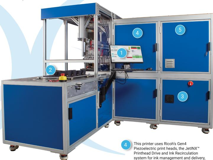
Media can be loaded into the shuttle during the print cycle, which saves time and contributes to the overall speed of the system.
